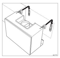
Hang the range hood in position using the adjustable brackets.
